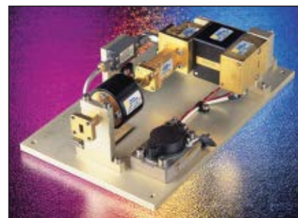
▲ Fig. 10 Farran's single-channel Ka-band downconverter with discrete waveguide components (approx. 125 x 250 x 75 mm) circa 1990.
